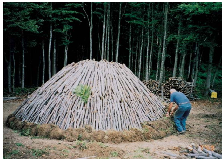
Le Banditacce ("Il Passeggere" Farm- 11 August 1999). Setting up a charcoal burner – phase one: the wood was arranged on two levels forming a cone shape. An aperture was left in the centre to act as a chimney. It was then carefully covered with pieces of turf. (Photograph by Leandro Gualtieri).
